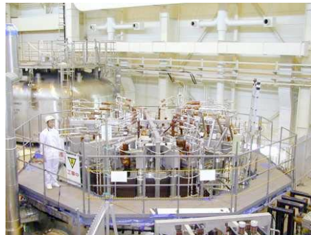
Largest High-Field Superconducting Magnet is World: 640 MJ and 13T!
