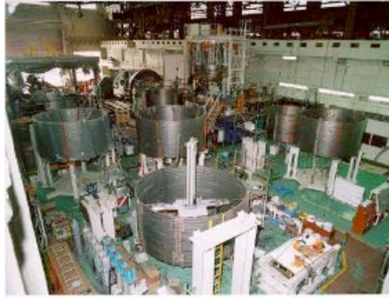
Largest High-Field Superconducting Magnet is World: 640 MJ and 13T!
