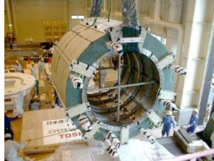
Largest High-Field Superconducting Magnet is World: 640 MJ and 13T!
